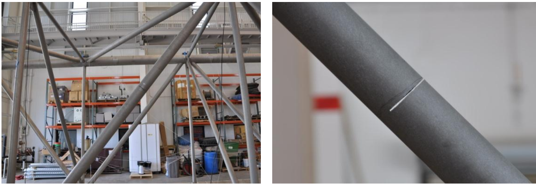
Figure 3.16: 90% cut at back panel diagonal at bay 9 (damage case 2).
