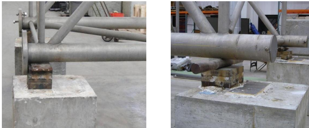
Figure 3.4: Boundary condition of experimental setup.
